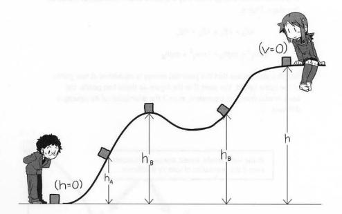
Since v = 0 at the highest height, the initial potential energy the box has is equal to all its mechanical energy. But we also know that the potential energy at point h is mgh, so we could express that as:
