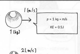
BUT, IN THE CASE OF KINETIC ENERGY, THE VALUE FOR THE FIRST BALL IS  $\frac{1}{2} \times 1 \text{ KG} \times (1 \text{ M/S})^2 = 0.5\text{J.}$  FOR THE SECOND BALL...
